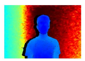
**3D imaging:** By measuring depth, a PAD system can differentiate between the contours of a live face and a 2D spoof.
