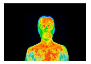
**Thermal imaging:** All objects emit heat, and as a result, exhibit an infrared signature. Since humans and synthetic materials emit significantly different amounts of heat, this approach can be used to determine wheter the object being presented is authentic.
