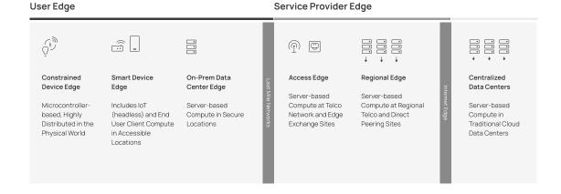
The Internet of Things (IoT) refers to all devices connected to the internet that can communicate with each other; this is the smart device edge in LF Edge parlance. There are also devices in the "constrained device edge" which may be connected via private networks or protocols other than TCP/IP and may even have intermittent connectivity.
