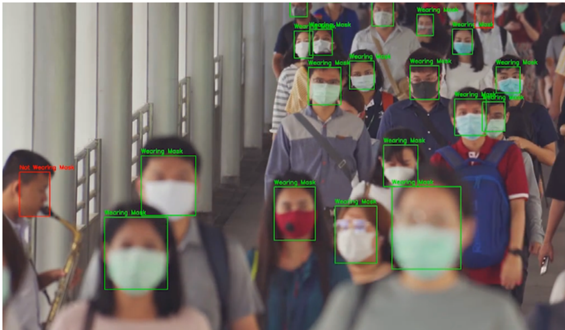
Figure 2 - Paravision's object detection algorithm detecting face masks in a crowd. Red = No mask; Green = Mask
